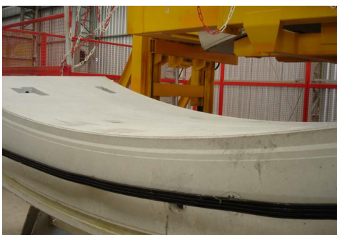
EPC BarChip synthetic fibre reinforced precast segmental tunnel lining
